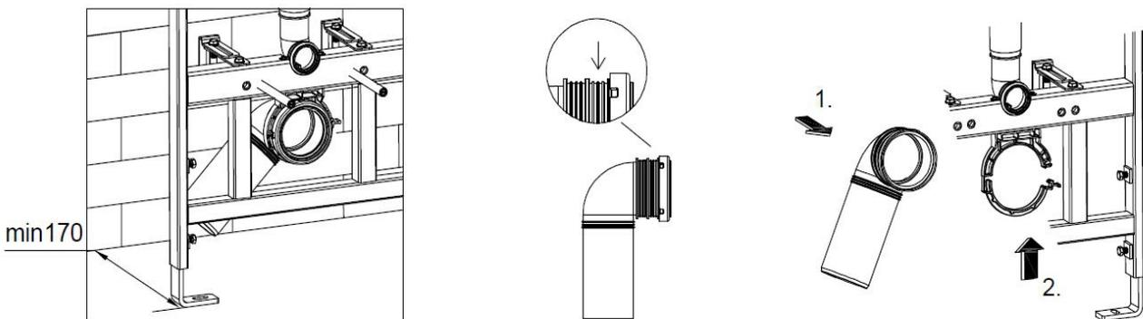
Below show the fixing width dimensions for the wall and floor screws, and the distance from the centre of the pan connector.
