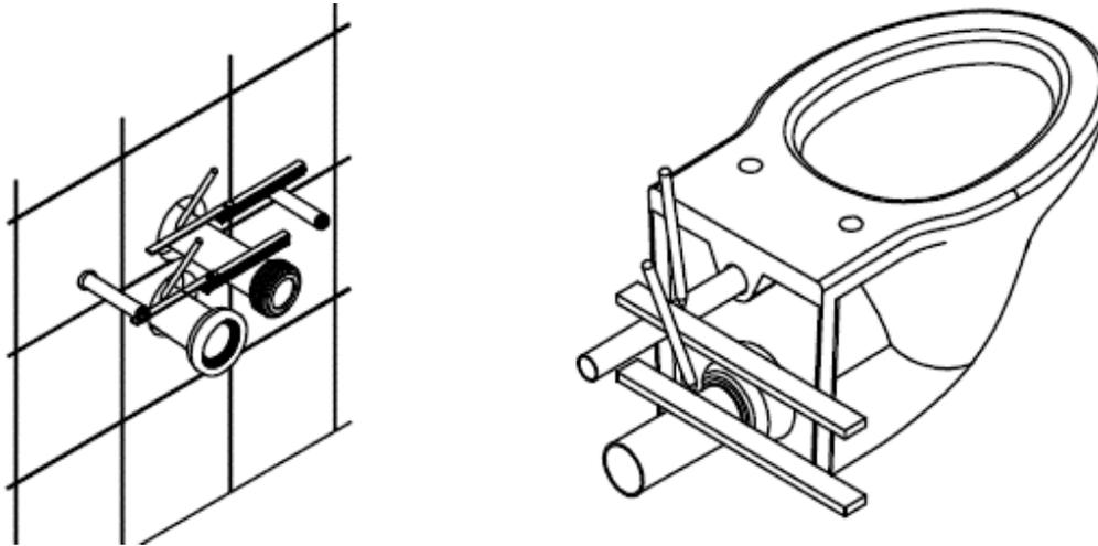
10. Remove from the frame and connect them to the flush hole and waste spigot on the rear of the toilet pan (Apply a small amount of washing up liquid to assist).
