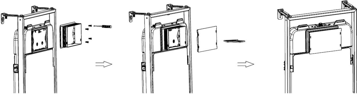
2. Push on the flush pipe and pan connector covers.
