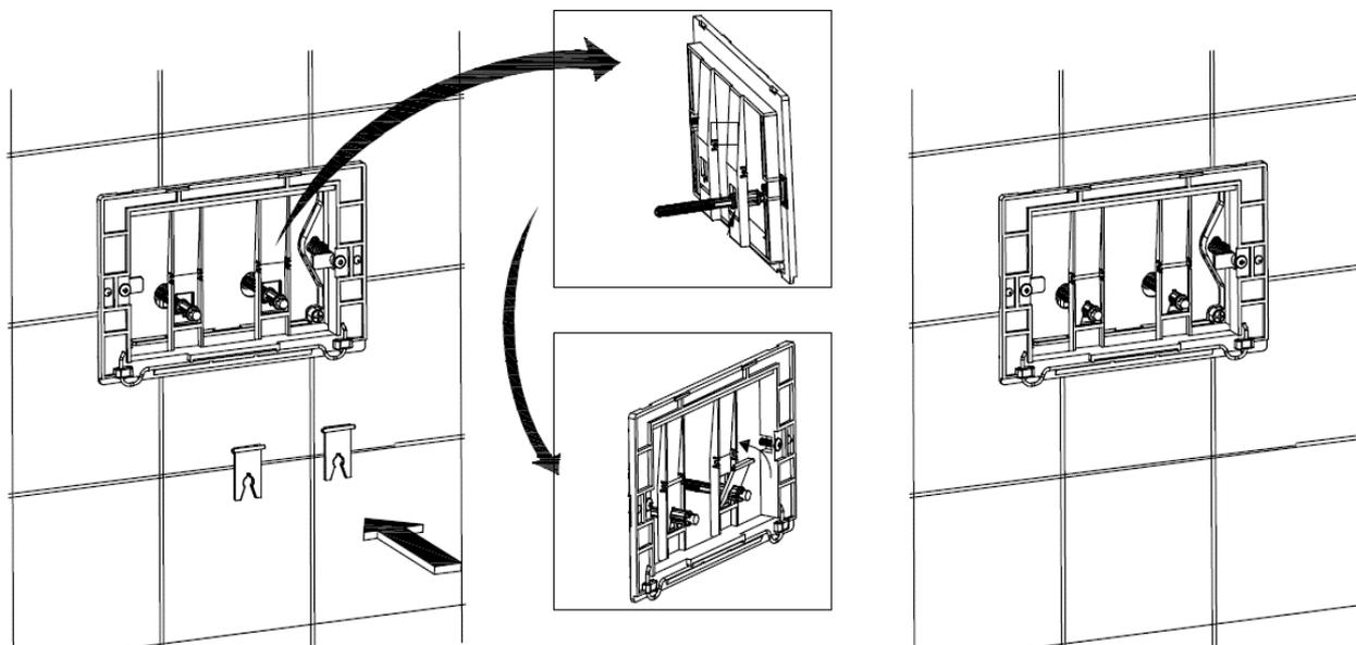
6. Attach the flush plate and click into position.
