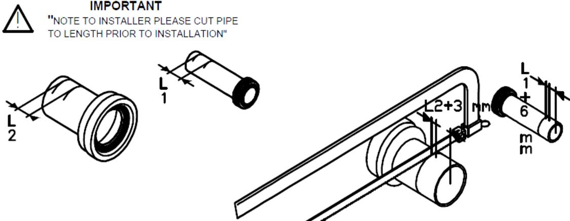
12. Prepare the flush pipe and pan connector ends removing any rough edges and create a small chamfer.
