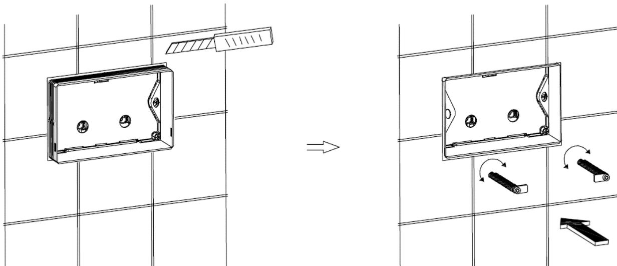
3. Secure the flush plate bracket to the fixing rods and secure using the screws provided.
